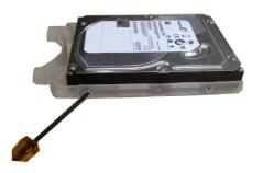
2. Use the screwdriver to fix the handle on the HDD.
