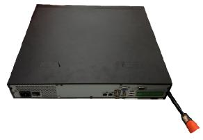
Use the screwdriver to loose the screws of the rear panel and then remove the front cover.
