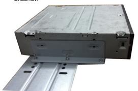
☐ Install SATA burner. Line up the SATA burner to the hole positions.
